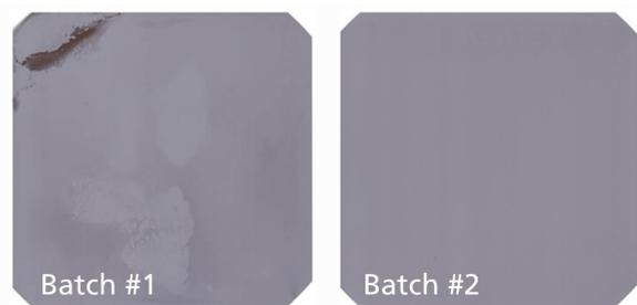
Figure 3: Two different wafer batches after different pre-cleaning processes. Batch #1 with visible stains and batch #2 without stains.
